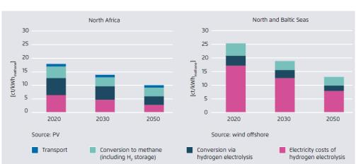
Comparison of the generation and transport costs of e-methane in North Africa (photovoltaic) and in the North and Baltic Seas (offshore wind)
