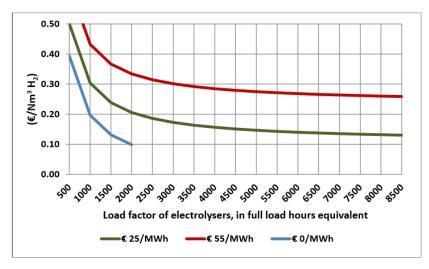
Assumptions: Capex electrolysers USD 450/kWin+30% installation +20% Opex; lifetime 30y; Weighted average capital cost 7%; efficiency 70%.
