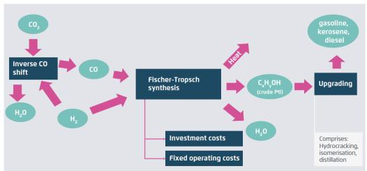
*Figure 11.* Liquid fuel production via Fischer-Tropsch synthesis
