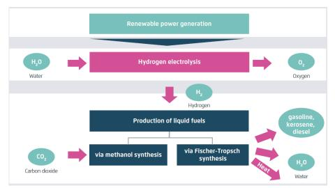
*Figure 9.* Main processes to synthetize e-liquid fuels
