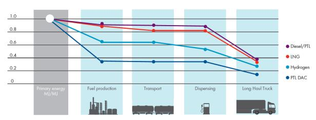
*Figure 19.* Cumulated fuel-powertrain efficiency for heavy duty vehicles
