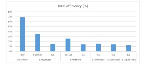
Figure 17. E-fuels final efficiency in engines (WTW approach)
