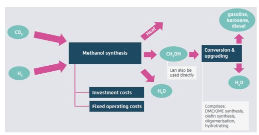
Figure 10. Liquid fuel production via methanol synthesis
